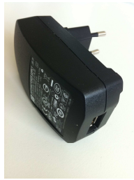
PSU for battery charging
