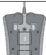
**Note:** Take care to have sufficient available length of cable in order to remove the terminal from its base and to unplug the connector. The serial cable can go under the base to reach the opening. Maybe by the way mentioned as (3), or right in front of the connectors mentioned as (1). Make an 18 mm diameter hole in the base in order to have a path for the squared angle connector. (14mm diameter is sufficient in case of base thickness lower than 4 mm)
