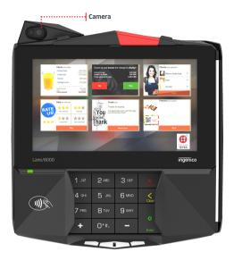
The Lane/8000 can be equiped with a module integrating a 5 megapixels autofocus camera. *Reference of the module : MODU/8005 WiFi/BT*
