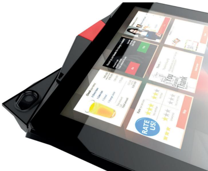
The Lane/8000 can be equipped with a module integrating a 5 megapixels autofocus camera.
