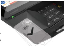
Your contactless terminal provides four contactless status lights located above the contactless logo.
