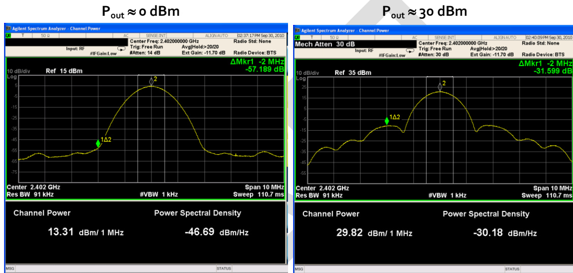
Figure 6. Spectral Shape—Linear and Compressed
