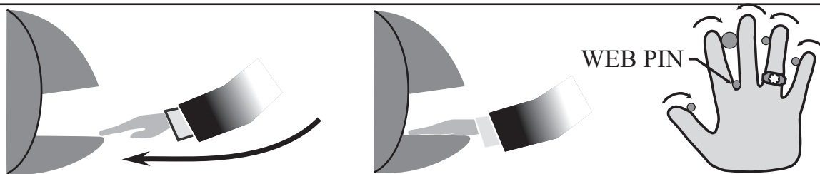
Figure 8-2: Placing Your Hand on the Platen
