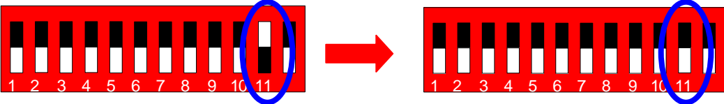
Fig. 27 DIP Switch (Uplink Path Activation)
