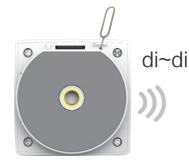
Enter the password for the Wi-Fi which the mobile phone is currently using, then turn up the volume on your phone and place it next to the device to add the camera.
