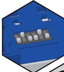
Control Switches allow you to choose how the Spider reacts when the sensors are activated. There are 64 different programming options!
