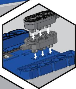
The motors and sensors each have snap connectors that attach to the Brain for both input and output!
