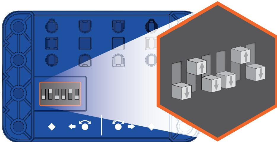
By changing the position of each Control Switch, you control how the Strandbeast reacts when the sensors are activated!
