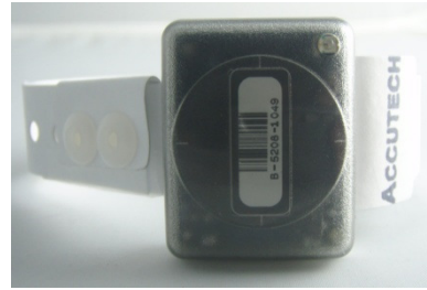
Figure 3.21 Secure the snap band by folding over the female snaps onto the male snaps. Carefully cut any excess band length material. Using an S-TAD activate the Tag.
