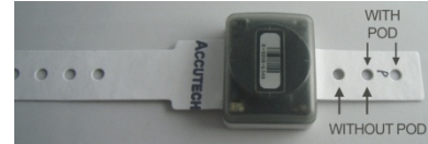
Figure 3.19 Slide the snap band through the Tag slot. Determine which holes to use (with or without pod)
