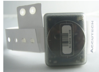
Figure 3.20 Determine band length needed and select holes. Position the coupon.
