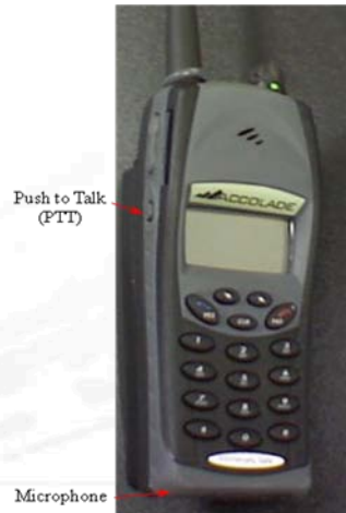
Fig. 4 Push-To-Talk and Microphone
