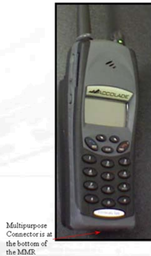
Fig. 6 Multi Purpose Connector (MPC)
