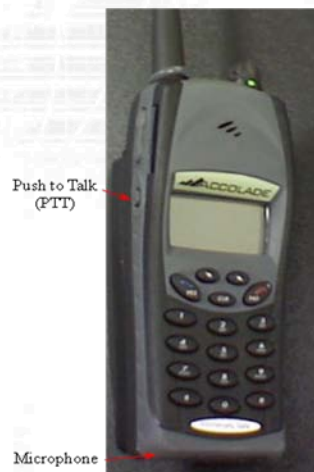
Fig. 7 Push-To-Talk and Microphone
