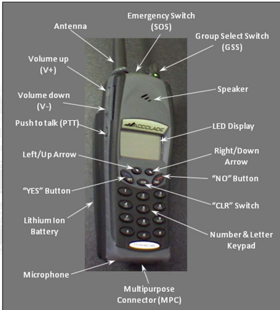
Figure 1: Handset and Location of Primary Features and Controls
