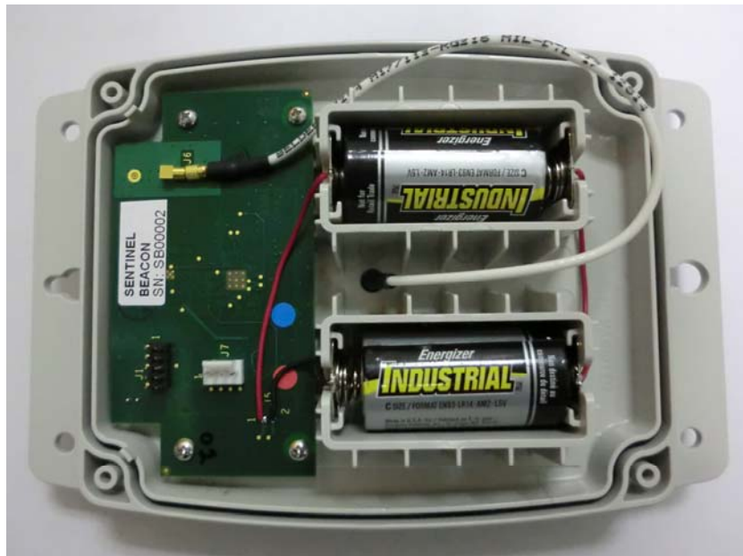
FIGURE 2: POWERING THE SENTINEL BEACON (SHOWN WITH BATTERIES INSTALLED)
