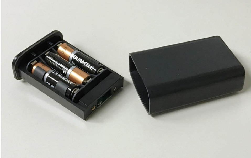
Figure 4 - Replace batteries and note proper polarity
