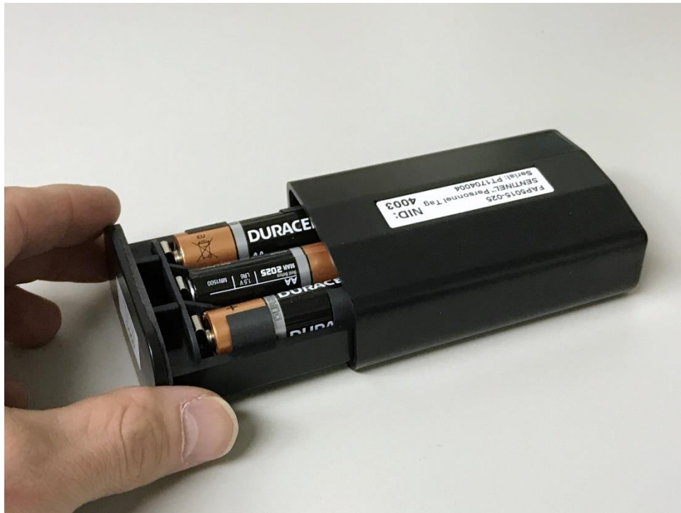
Figure 3 - Carefully slide out interior tray
