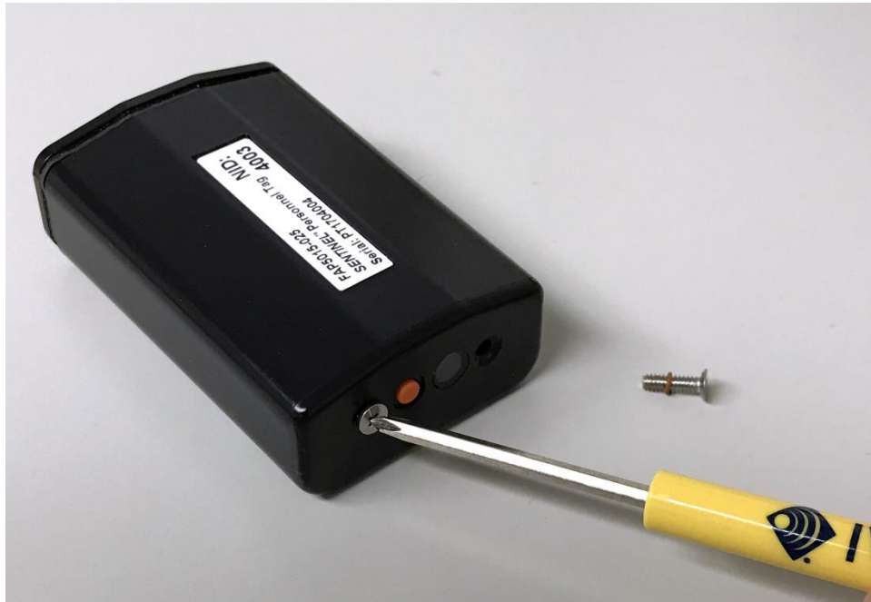
Figure 2 - Remove screws with Phillips screwdriver
