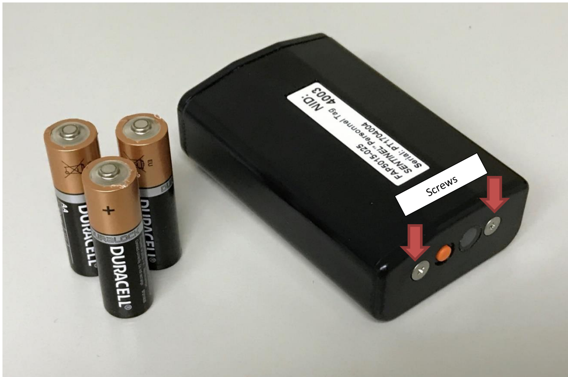
Figure 1 - Enclosure is held together by two screws
