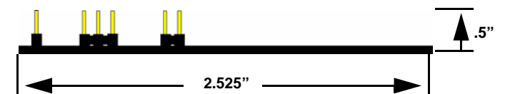
Figure 4 E*1941 One-Way Binary RF Module Dimensions
