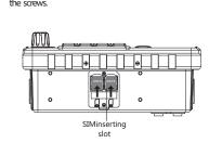
Insert the SIM card, cover on the SIM holder and tighten
