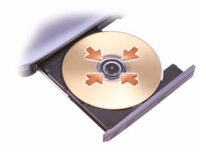
**3** Place the disc, label side up, in the center of the tray and snap the disc onto the spindle.
