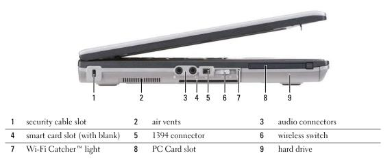
**SECURITY CABLE SLOT** — Lets you attach a commercially available antitheft device to the computer (see "Security Cable Lock" on page 67).
