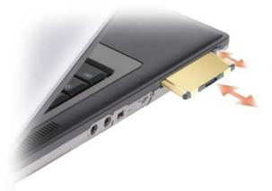
The computer recognizes most PC Cards and automatically loads the appropriate device driver. If the configuration program tells you to load the manufacturer's drivers, use the floppy disk or CD that came with the PC Card.
