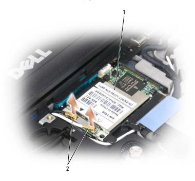
1 WLAN card 2 antenna cables (2)
