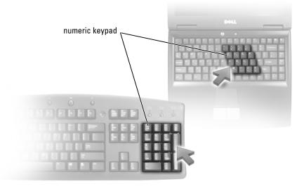
The numeric keypad functions like the numeric keypad on an external keyboard. Each key on the keypad has multiple functions. The keypad numbers and symbols are marked in blue on the right of the keypad keys. To type a number or symbol, hold down  $\langle Fn \rangle$  and press the desired key.
