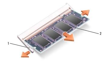
1 securing clips (2 per connector) 2 memory module
