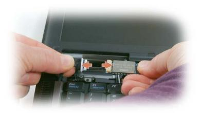
**6** Disconnect the card from the cable and remove the card from the computer.
