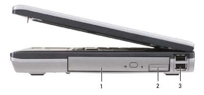
1 optical drive in media bay 2 media-bay device latch release 3 USB connectors (2)
