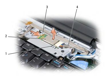
securing tab 1 card securing tab cable
