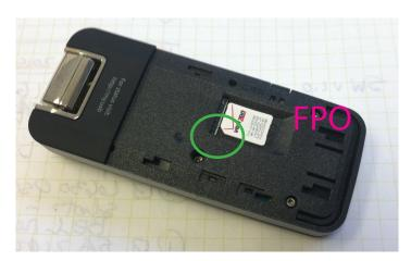
**3** Gently push the 4G LTE SIM Card forward until the spring catches and the card remains securely in the slot.
