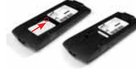
3. Gently push the SIM card forward until the spring catches and the card remains securely in the slot.
