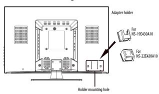
**2** Place the AC power adapter into the holder.
