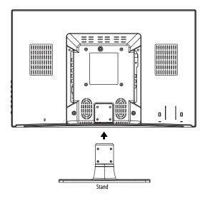
**6** Secure the stand with the four provided screws.
