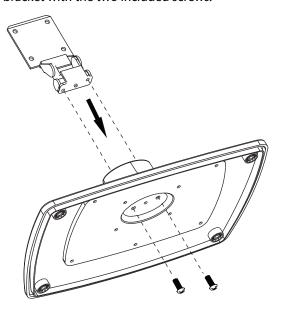
2 Install the bracket cap on top of the bracket.
