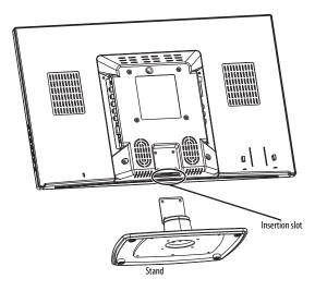
5 Slide the stand into the insertion slot.
