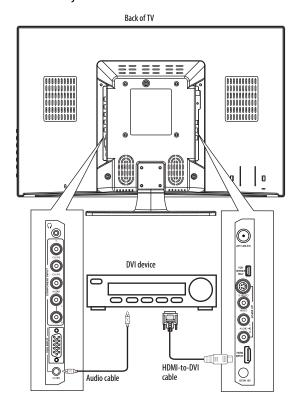
3 Connect an audio cable to the VGA AUDIO INPUT jack on the back of your TV, then connect the other end of the cable into the AUDIO OUT jack on the DVI device.
