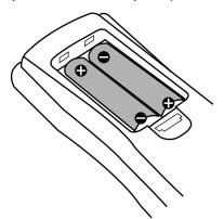
**3** Press down on the battery compartment cover until it clicks into place.
