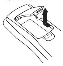
2 Insert two AAA batteries into the battery compartment. Make sure that you match the + and – symbols on the batteries with the + and – symbols in the battery compartment.
