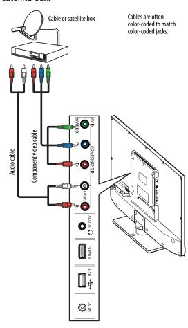
4 Connect an audio cable (not provided) to the L/R AUDIO jacks on the side of your TV and to the audio out jacks on the cable or satellite TV box.
