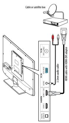
5 Connect a 3.5mm audio cable (not provided) to the AUDIO jack on the side of your TV and to the AUDIO OUT jacks on the cable or satellite box.
