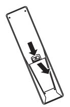
2 Insert two AAA batteries into the battery compartment. Make sure that you match the + and – symbols on the batteries with the + and – symbols in the battery compartment.
