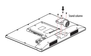
**3** Secure the base to the stand column using the four long screws (provided).
