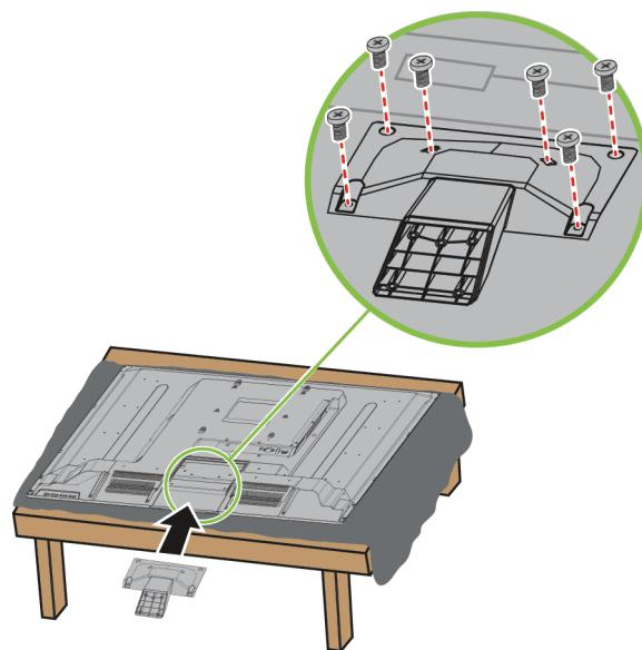
**3** Secure the TV stand to the stand column with the five provided 18 mm screws (the longer screws).
