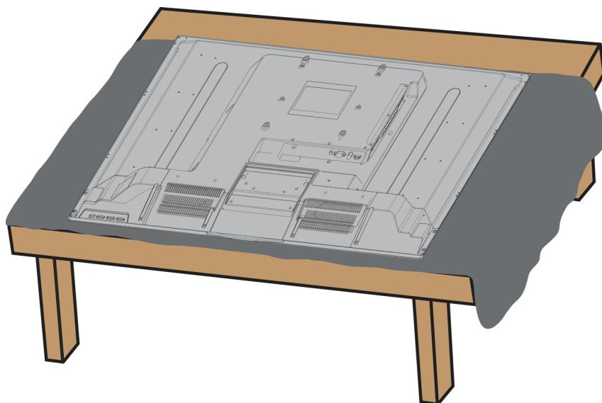
**2** Secure the stand column to your TV with the six provided 16 mm screws (the shorter screws).
