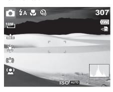
3 Press the shutter button halfway. The camera automatically adjusts the focus and exposure. When the camera is ready to take the photo, the focus bracket turns green, and the aperture value, shutter speed, and ISO setting are displayed.
