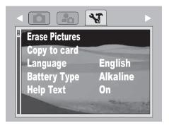
4 Press ▼ or ▲ to highlight Battery Type, then press right ▶ or OK/DISP to select it.
