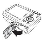
3 Insert two AA batteries into the battery compartment. Make sure that you match the + and – symbols on the batteries with the + and – symbols in the battery compartment.
