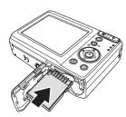
To remove the memory card, push the card in slightly to release it, then pull the card out of the card slot.
