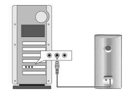
3 Plug the black plug from the AC adapter into the back of the right speaker and the other end into a wall outlet or power strip.
