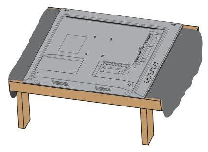
**2** Find the front of the left and right TV stands. Secure the stands to your TV using the two provided  $M4 \times 14$  mm screws.
