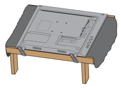
2 If the stands are attached, remove the two screws that secure the stands to the TV, then remove the stands.
