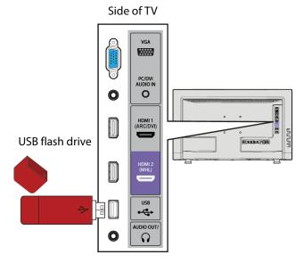
1 Plug a USB flash drive into the **USB** port on the side of your TV.
