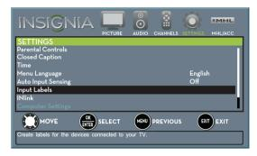
3 Press ▲ or ▼ to highlight Input Labels, then press ENTER. The SETTINGS · INPUT LABELS screen opens with the input source field highlighted.
