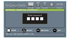
**4** Press the number buttons to enter the four-digit password. The SETTINGS · PARENTAL CONTROLS menu opens.
