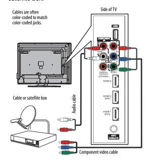
4 Connect an audio cable (not provided) to the L/R AUDIO jacks on the side of your TV and to the audio out jacks on the cable or satellite TV box.
