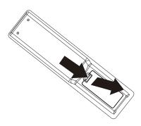
2 Insert two AAA batteries into the battery compartment. Make sure that you match the + and – symbols on the batteries with the + and – symbols in the battery compartment.
