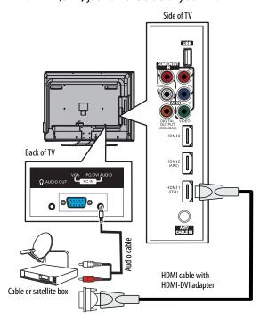
5 Connect a 3.5mm audio cable (not provided) to the PC/DVI AUDIO jack on the back of your TV and to the AUDIO OUT jacks on the cable or satellite box.
