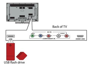
1 Plug a USB flash drive into the **USB** port on the back of your TV.
