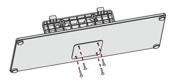
**3** Carefully place your TV facedown on a soft, cushioned surface to protect the screen from damages and scratches.
