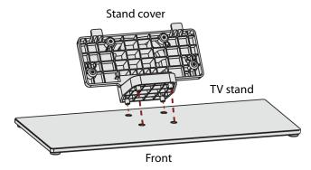
2 Secure the stand cover to the TV stand with the four provided  $ST4 \times 16$  mm screws (the long screws).
