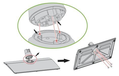
2 Secure the column to the stand with three of the provided M5  $\times$  12 mm screws.
