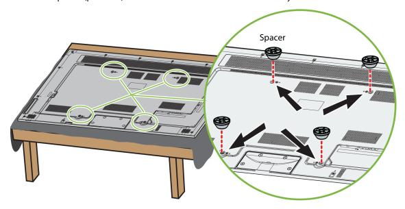
3 Attach the wall-mount bracket to your TV using either the four provided  $M6 \times 30$  mm screws or the screws that came with the wall-mount bracket. See instructions that came with the wall-mount bracket for information about which screws to use and how to correctly hang your TV.
