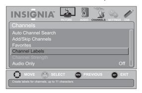
3 Press ▲ or ▼ to highlight **Channel Labels**, then press **ENTER**. The *CHANNELS-Channel Labels* screen opens with the channel number field highlighted.
