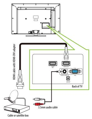
5 Connect a 3.5mm audio cable (not provided) to the PC/DVI AUDIO IN jack on the back of your TV and to the AUDIO OUT jacks on the cable or satellite box.
