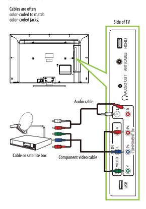
4 Connect an audio cable (not provided) to the COMPONENT IN L/R audio jacks on the side of your TV and to the audio out jacks on the cable or satellite TV box.
