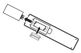
2 Insert two AAA batteries into the battery compartment. Make sure that you match the + and – symbols on the batteries with the + and – symbols in the battery compartment.
