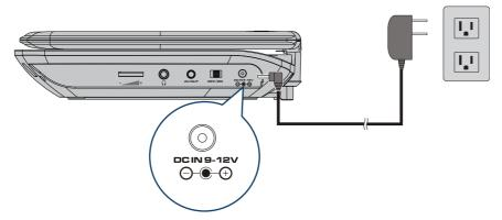
2 Plug the other end of the adapter into an AC wall outlet.
