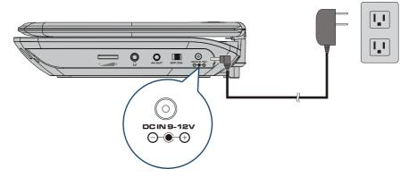
When the battery is charging, the battery charge indicator lights red. When the battery is fully charged, the charge light turns yellow.
