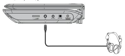
For two headphones, plug each headphone (not included) into the included y-cable, then plug the y-cable into the (headphone) jack.
