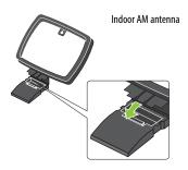
5 To connect the Indoor AM antenna, press the GND and AM Loop levers, insert the ends of the wires, then release the levers. Make sure that only the bare, stripped wire is inserted in the jack.
