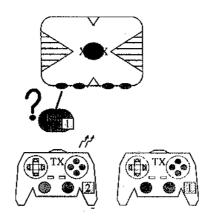
First press CONNECT key of receiver, then press the CONNECT key of your wished controller. After that, ID resetting has completed. At the same time, channel will confirm and CONNECT LED lights. So you can play normally.
