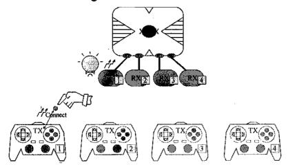
Turn on the next controller power and press CONNECT key, so this channel will confirm and CONNECT LED lights. In this way you can reset the rest channels in turn.
