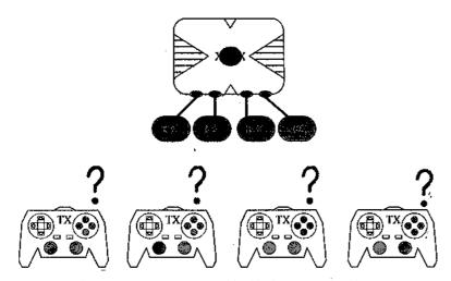
In this situation, please turn off all the controllers power, Then turn on one of controller power and press CONNECT key. So new channel will confirm and Connect LED lights.
