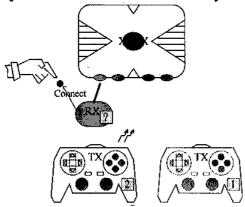
Step 2: Press the CONNECT key of controller.
