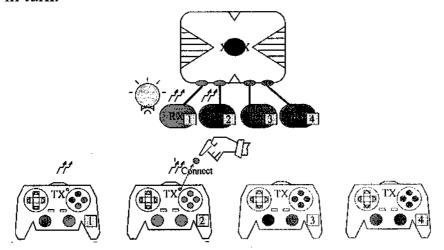
c). In the situation that receiver's ID is different from controller's Controllers' original setting have one for one ID. When receiver's original ID is different from controller's, you'd better reset ID.
