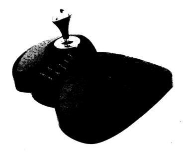
USA & CANADA: www.inteclink.com EUROPE: www.inteclinkeurope.com MODE BUTTON & LED INDICATOR: Use to change mode selection (digital or analog). The LED indicator will illuminate in analog mode, and will not illluminate in digital mode.
