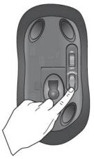
Press Connect button on receiver. Then press Connect button on buttom of mouse.
