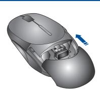
English To readily carry the mouse: (a) Open the battery case. (b) Insert nano wireless receiver inside the compartment by the direction of the arrow. (c) Close the battery case back.
