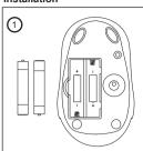
On the underside of the mouse. open the battery compartment, insert the batteries in the compartment in the direction shown and replace the cover
