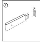
Insert the wireless receiver in one of your PC's USB ports. With vour PC switched on, follow the device installation wizard to complete the installation of the new LISB device
