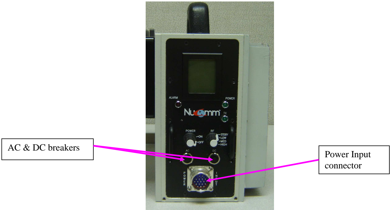
Figure 4: Input Power & Breakers location
