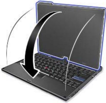
4. Press the center latch down to lock the display.
