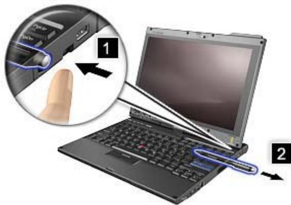
**\* Note:** The pen contains pressure sensors. Do not push the tip of the pen for an extended period of time. Do not subject the pen to shock or vibration.
