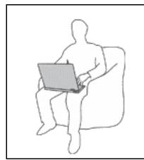
When your computer is turned on or the battery is charging, the base, the palm rest, and some other parts may become hot. The temperature they reach depends on the amount of system activity and the level of charge in the battery.
