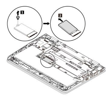
6. Insert the new M.2 solid-state drive into the slot at an angle of about 20 degrees **■**. Pivot the M.2 solid-state drive downward **■**. Install the screw to secure the M.2 solid-state drive **■**.
