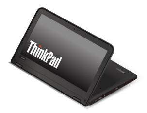
In the stand mode, the keyboard and the touch pad are automatically disabled. However, you can control some functions of your computer through the multi-touch screen, without the use of the keyboard and the touch pad. For more information, see "Using the multi-touch screen" on page 21.
