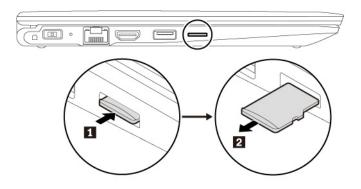
3. Insert the new card into the microSD card slot. The card might stop before it is installed into the card reader. Ensure that you insert the card firmly until you hear a click.
