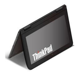
In the tent mode, the keyboard and the touch pad are automatically disabled. However, you can control some functions of your computer through the multi-touch screen, without the use of the keyboard and the touch pad. For more information, see "Using the multi-touch screen" on page 21.
