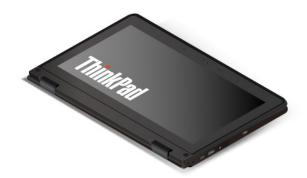
In the tablet mode, the keyboard and the touch pad are automatically disabled. However, you can control some functions of your computer through the multi-touch screen, without the use of the keyboard and the touch pad. For more information, see "Using the multi-touch screen" on page 21.
