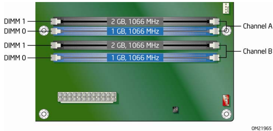
Figure 16. Example Dual Channel Memory Configuration with Four DIMMs
