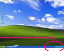
If the icon can not be found, go to the control panel from the system menu and double click the C-Media CPL icon. Open "CMI Audio Config" and then go to "Information" tab. Make sure "Show the audio configuration icon in the system tray" is checked.
