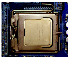
Fig. 4 Once the CPU is properly inserted, please replace the load plate and push the metal lever back into its original position.
