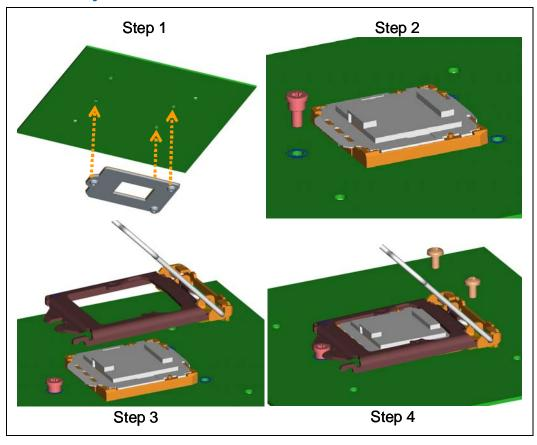
**Note:** Here ILM assembly shown in figure is without ILM cover preinstalled.
