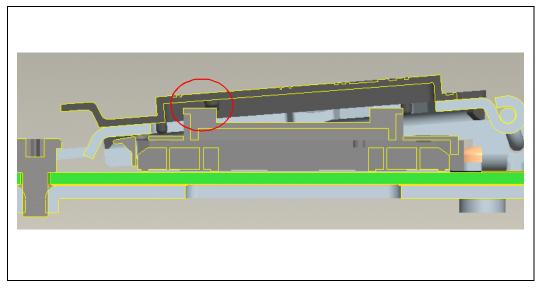
As indicated in Figure 4-7, the pick and place cover cannot remain in place and used in conjunction with the ILM Cover. The ILM Cover is designed to interfere and pop off if the pick and place cover is unintentionally left in place. The ILM cover will also interfere and pop off if the ILM is closed with a processor in place in the socket.
