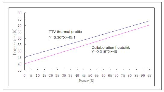
Table 9-2. Comparison between TTV Thermal Profile and Thermal Solution Performance for Intel® Xeon® Processor E3-1280 (95W) (Sheet 1 of 2)
