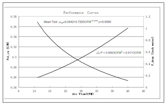
This 1U Reference thermal solution  $\Psi$ ca(mean+3sigma) is computed to 0.353°C/W at the airflow of 15.5 CFM, which just meets Intel® Xeon® processor E3-1280 (95W) TTV thermal profile specification when  $T_{IA}$  is 40 °C.
