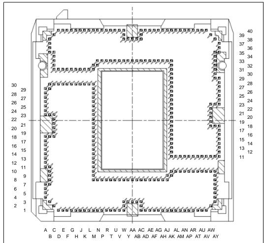
Figure 3-2. LGA1155 Socket Contact Numbering (Top View of Socket)
