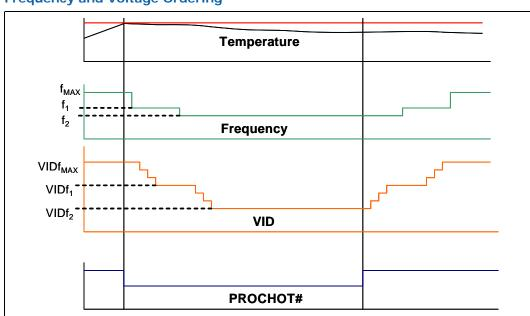
Figure 6-7. Frequency and Voltage Ordering
