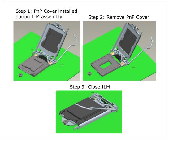
As indicated in Figure 4-6, the pick and place cover should remain installed during ILM assembly to the motherboard. After assembly, the pick and place cover is removed, and the ILM mechanism (with the ILM cover installed) closed to protect the contacts. The ILM Cover is designed to pop off if the pick and place cover is accidentally left in place and the ILM closed with the ILM Cover installed. This is shown in Figure 4-7.
