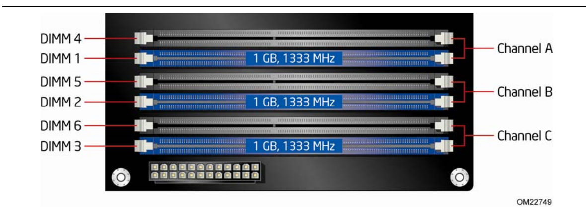
Figure 15. Example Configuration Using Three DIMMs
