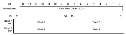
*Note:* For active 16 bits per pixel operation, the Raw Pixel Data is sent directly to the LCD panel pins and must be in the same format as required by the LCD panel.
