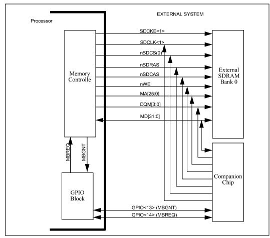
Figure 6-31. Alternate Bus Master Mode
