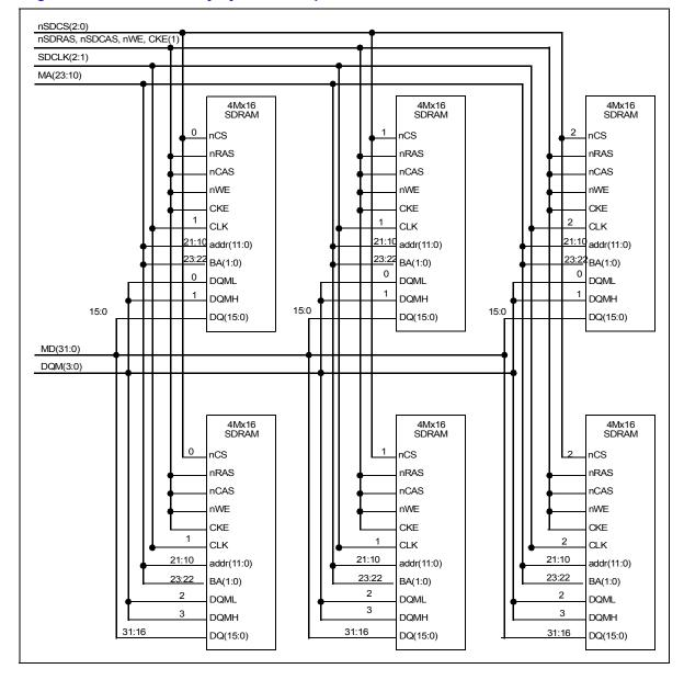
Figure 6-2. SDRAM Memory System Example
