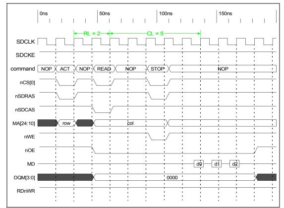
Figure 6-12. SMROM Read Timing Diagram Half-Memory Clock Frequency
