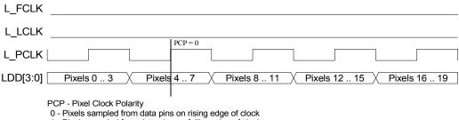
1 - Pixels sampled from data pins on falling edge of clock
