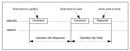
Figure 15-3. MMC Mode Operation With Data Token
