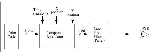
This dithering concept is applied separately to each color displayed. Each color has zeros added to make the data for each color 8 bits. If a monochrome display is used, only a single matrix (blue) is used.
