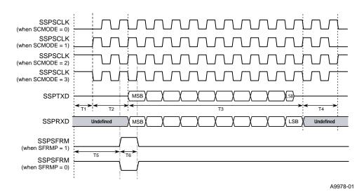
If the SSP is a master to frame, SSPTXD is Hi-Z two clock edges after the clock edge that drives the LSB. This occurs even if the SSP is a master of clock and this clock edge does not appear on the SSPSCLK. Figure 16-16 shows the pin timing for this mode.
