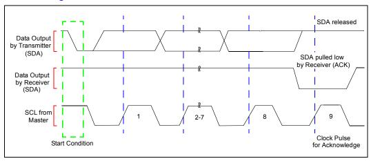
Figure 9-5. Acknowledge on the I<sup>2</sup>C Bus
