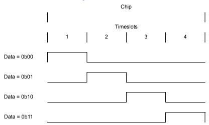
Figure 11-2. 4PPM Modulation Example
