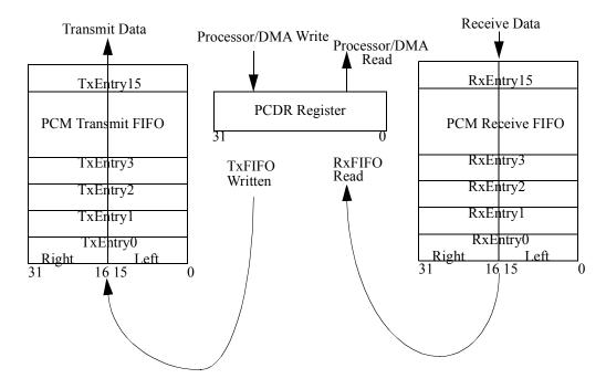
Figure 13-9. PCM Transmit and Receive Operation
