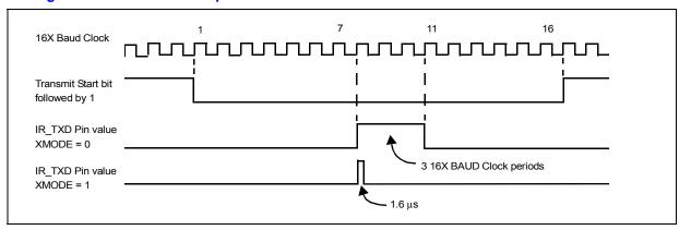
To prevent transmitter LED reflection feed back to the receiver, disable the IR receiver decoder when the IR transmit encoder transmits data and disables the IR transmit encoder when the IR receiver decoder receives data. The RCVEIR and XMITIR bits in the Infrared Selection Register (ISR) must not be set at the same time (refer to Section 17.5.15).
