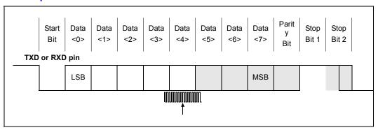
Receive data sample counter frequency is 16 times the value of the bit frequency. The 16X clock is created by the baud rate generator. Each bit is sampled three times in the middle. Shaded bits in Figure 10-1 are optional and can be programmed by software.
