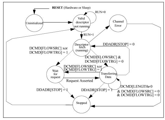
Figure 5-4. Descriptor Fetch Mode Channel State
