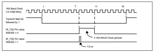
**Note:** Note: The SIR TXD output pin is automatically held deasserted when the RCVEIR bit is set. Before setting the RCVEIR bit, check that the TEMT bit is 1. While receiving, any data placed in
