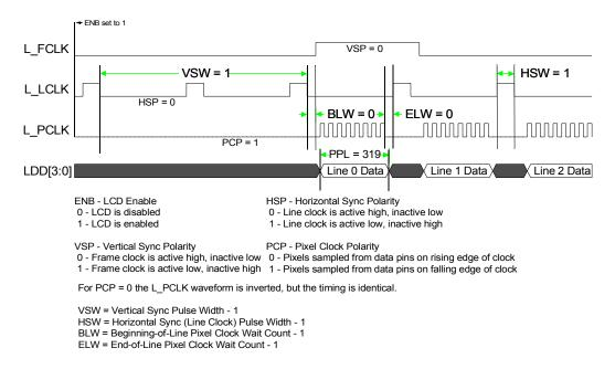
Figure 7-13. Passive Mode End-of-Frame Timing
