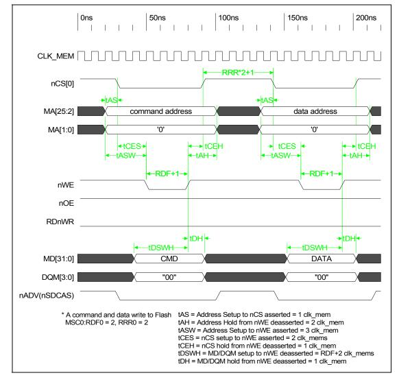
Figure 6-23. Asynchronous 32-Bit Flash Write Timing Diagram (2 Writes)
