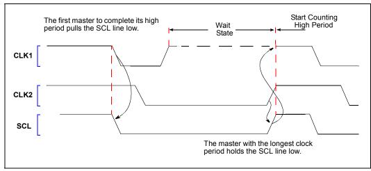
Figure 9-6. Clock Synchronization During the Arbitration Procedure
