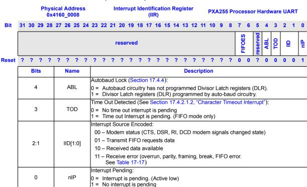
Table 17-9 shows the priority, type, and source of the Interrupt Identification register interrupts. It also gives the reset condition used to deassert the interrupts. Bits (0-3) of the IIR register represent priority encoded interrupts. Bits (4-7) do not.
