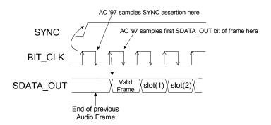
The SDATA\_OUT composite stream is MSB-justified (MSB first). The ACUNIT fills all non-valid slot bit positions with zeroes. If fewer than 20 valid bits exist in an assigned valid time slot, the ACUNIT stuffs all trailing non-valid bit positions of the 20-bit slot with zeroes.
