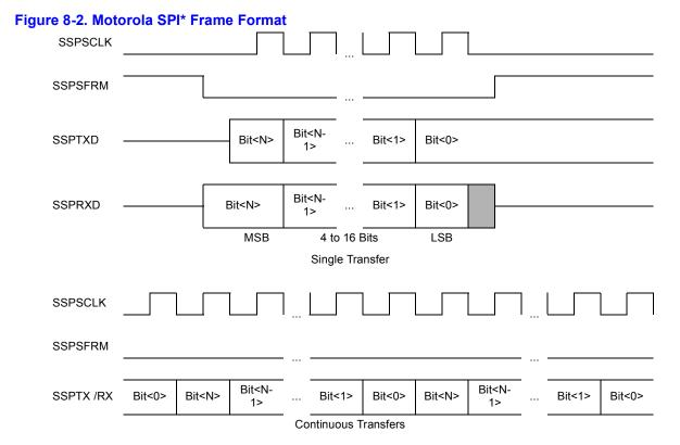
Note: SSPSCLK's phase and polarity can be configured for four modes. This example shows one of those modes.
