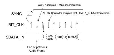
The SDATA\_IN composite stream is MSB justified (MSB first) and the AC'97 CODEC fills non-valid bit positions with zeroes. SDATA\_IN data is sampled on BITCLK's falling edge.
