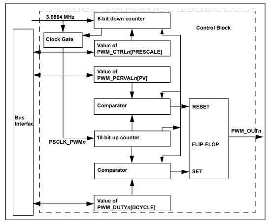
Figure 4-3. PWMn Block Diagram
