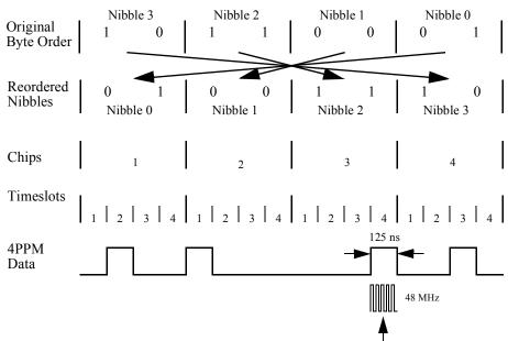
Receive data sample counter frequency = 6/pulse width. Each timeslot is sampled on the third clock.
