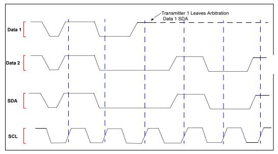
Figure 9-7. Arbitration Procedure of Two Masters
