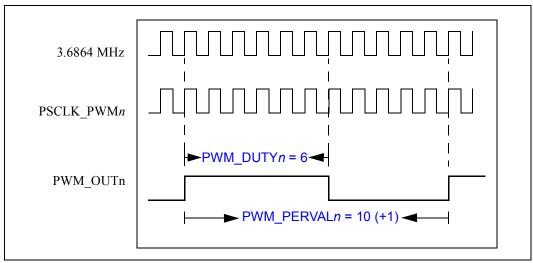
PWM\_PERVAL[PV] = 0xA PWM\_DUTY[FDCYCLE] = 0x0 PWM\_DUTY[DCYCLE] = 0x6 PWM\_CTRL[PRESCALE] = 0x0
