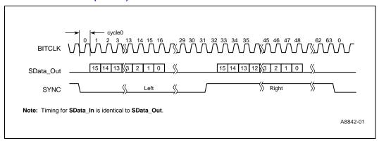
Figure 14-2. MSB-Justified Data Formats (16 bits
