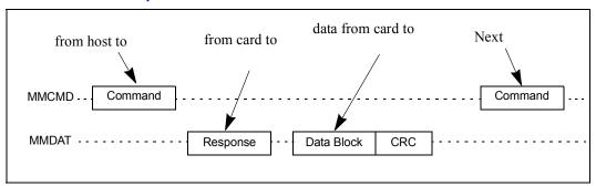
Figure 15-6. SPI Mode Write Operation
