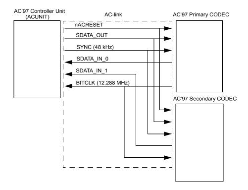
Figure 13-1. Data Transfer Through the AC-link
