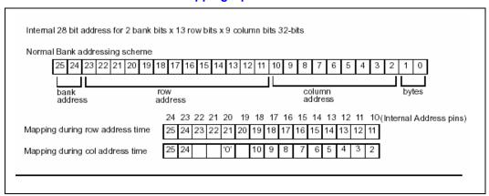
Table 6-7. External to Internal Address Mapping for Normal Bank Addressing (Sheet 1 of 3)
