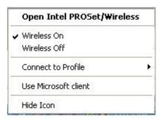
The Intel PROSet/Wireless icon displays in the task tray located in the lower right corner of your Windows desktop. Right-click the status icon to display the menu options. Intel PROSet/Wireless can support multiple adapters. These wireless adapters are displayed in the task tray menu options.
