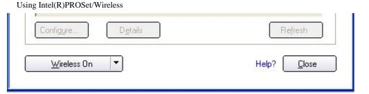
The Windows XP Wireless Zero Configuration feature provides a built-in wireless configuration utility. This feature can be enabled and disabled in Windows XP or by clicking **Use Microsoft Client** on the Tools menu. If XP Zero Configuration is enabled, the features in Intel PROSet/Wireless are disabled.
