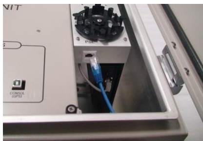
Figure 3-6 Power cable connection (PoE type)
