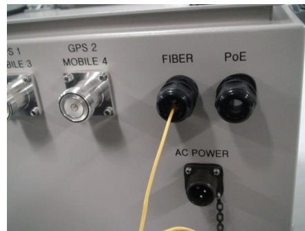
Figure 3-8 LC/UPC fiber connector connection
