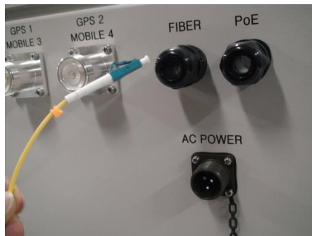
Figure 3-8 LC/UPC fiber connector connection
