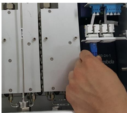
Figure 3-6 Power cable connection (PoE type)
